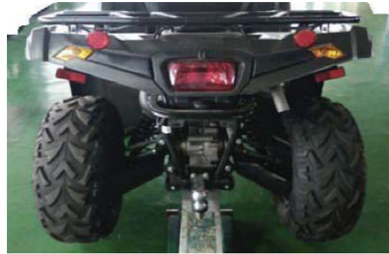
TYPICAL BACK UP POINT LOCATION
