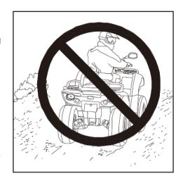
Never apply the rear brake while rolling backwards. Apply the front brake. When fully stopped, apply the rear brake as well, and shift the gear to parking.
