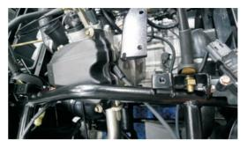
Spark plug cap, front cylinder
